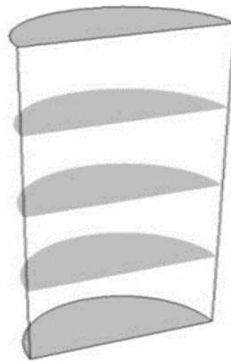
Fig. 4. Division of the dryer chamber into five plates
