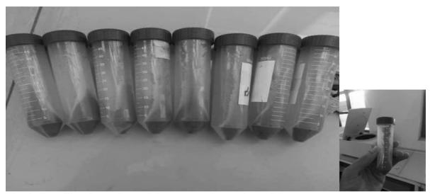
Fig. 1. Centrifuged samples and the separated cyanobacterial mat.
