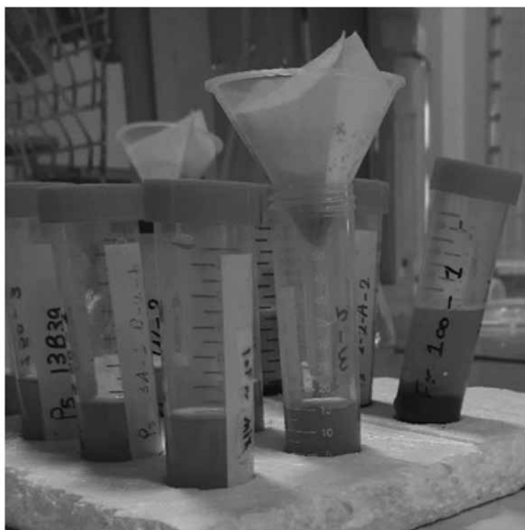
Fig. 2. Initial purification of the algal extract was performed using ordinary filter paper
